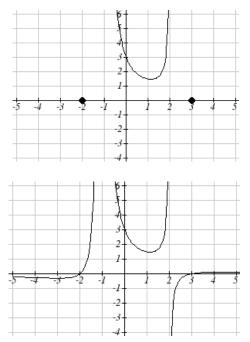
After passing through the horizontal intercepts, the graph will then level off towards an output of zero, as indicated by the horizontal asymptote.
