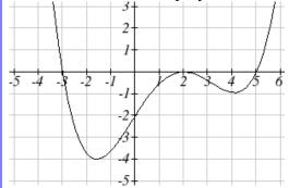
This graph has three horizontal intercepts: x = -3, 2, and 5. At x = -3 and 5 the graph passes through the axis, suggesting the corresponding factors of the polynomial will be linear. At x = 2 the graph bounces at the intercept, suggesting the corresponding factor of the polynomial will be  $2^{nd}$  degree (quadratic). Together, this gives us:  $f(x) = a(x+3)(x-2)^2(x-5)$
