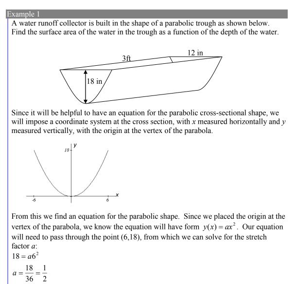
Our parabolic cross section has equation  $y(x) = \frac{1}{2}x^2$
