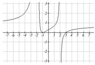
At the horizontal intercept x = 3 corresponding to the (x-3) factor of the numerator, the graph passes through the axis as we'd expect from a linear factor.
