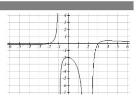
behavior similar to  $\frac{1}{x}$ , with the graph heading toward positive infinity on one side and heading toward negative infinity on the other. The asymptote at x = 2 is exhibiting a behavior similar to  $\frac{1}{x^2}$ , with the graph heading toward negative infinity on both sides of the asymptote.
