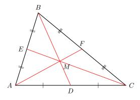
In the above, if  $\overline{AF}$ ,  $\overline{CE}$ , and  $\overline{BD}$  are medians of  $\triangle ABC$ , then they intersect at a single point, M, and  $\overline{CM}=2\overline{ME}$ ,  $\overline{AM}=2\overline{MF}$ ,  $\overline{BM}=2\overline{MD}$ .
